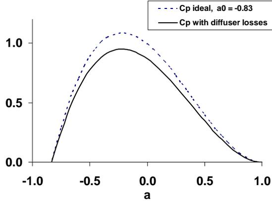
**Figure 4 Effect of diffuser inefficiency on power coefficient**
