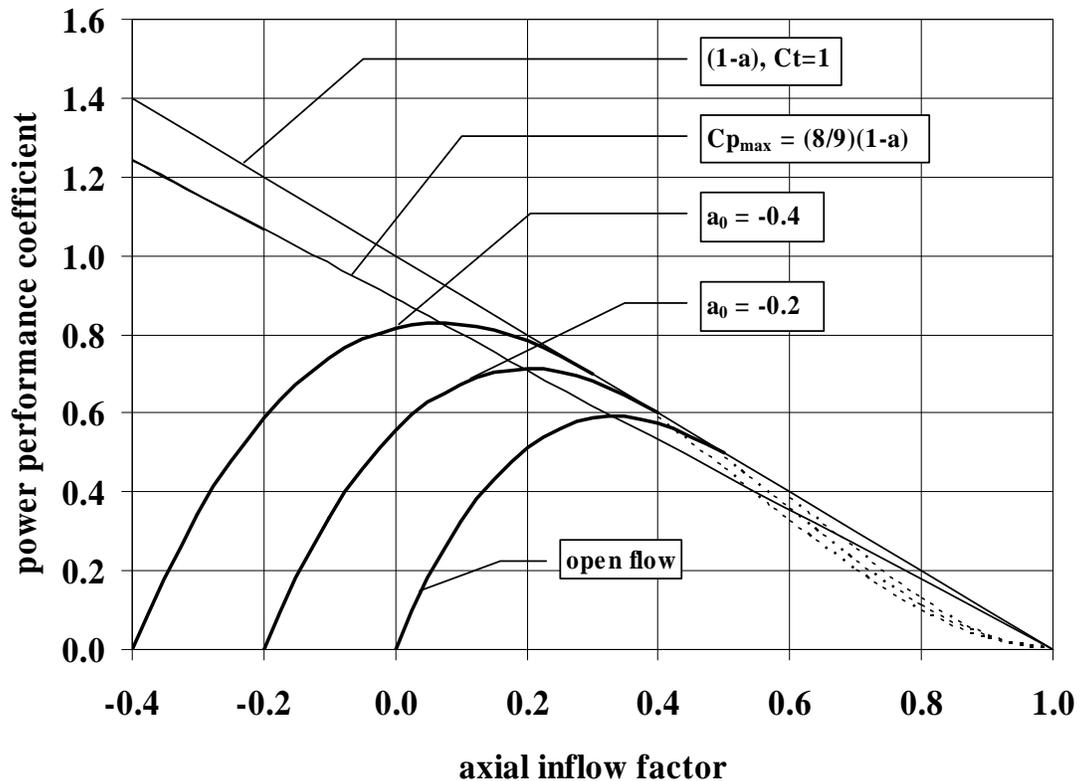
Figure 2 Limiting  $C_p$  characteristics
